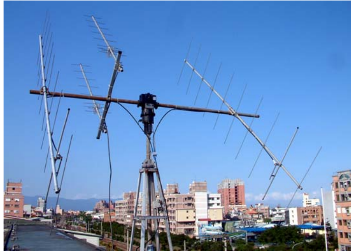
BX1AD 2 yagi array used on 70 cm EME
